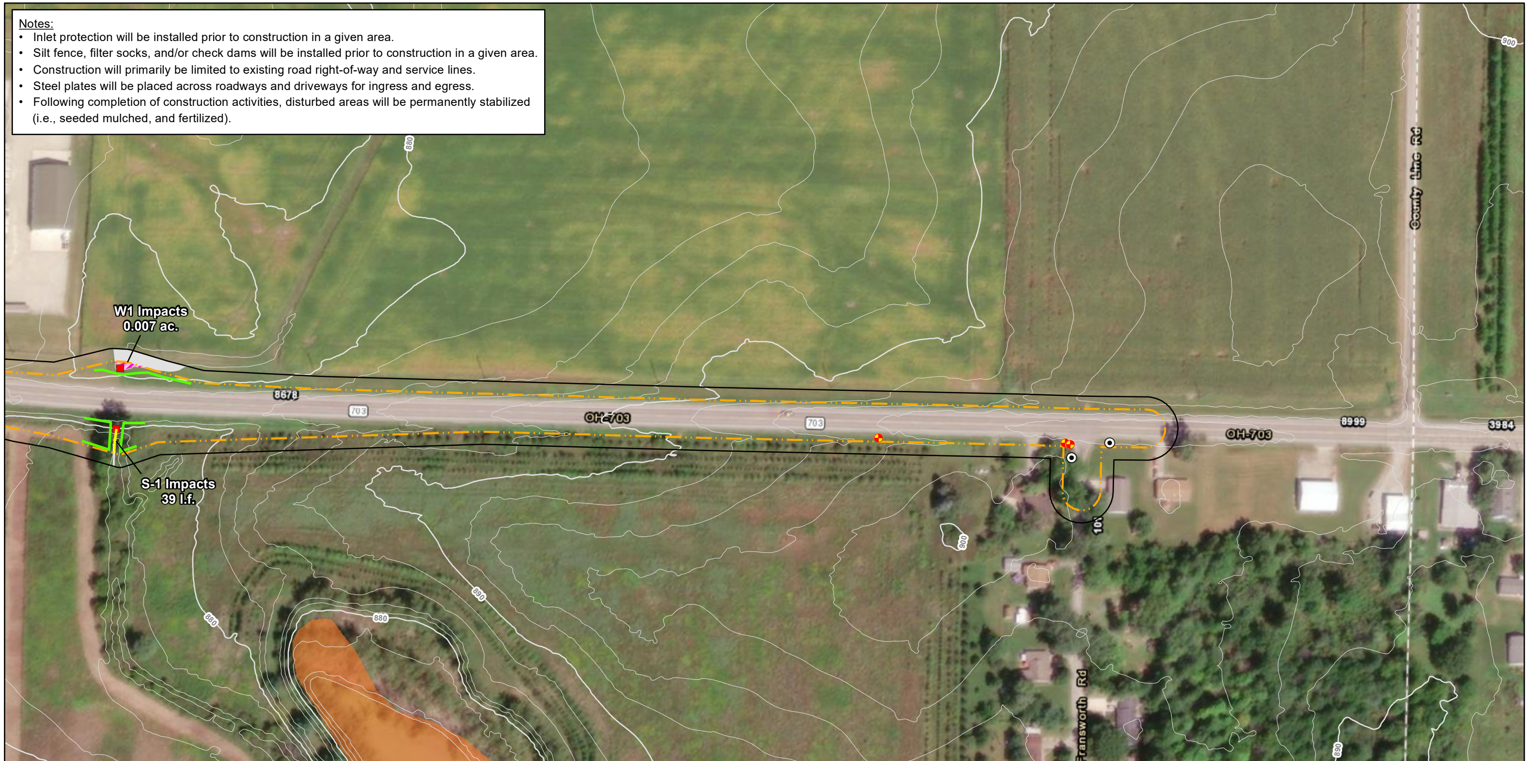
Figure C-1.02. SWPPP Map of Wetlands and Other Water Resources. PIR 2399 - Peach Tree S.R. 703.
