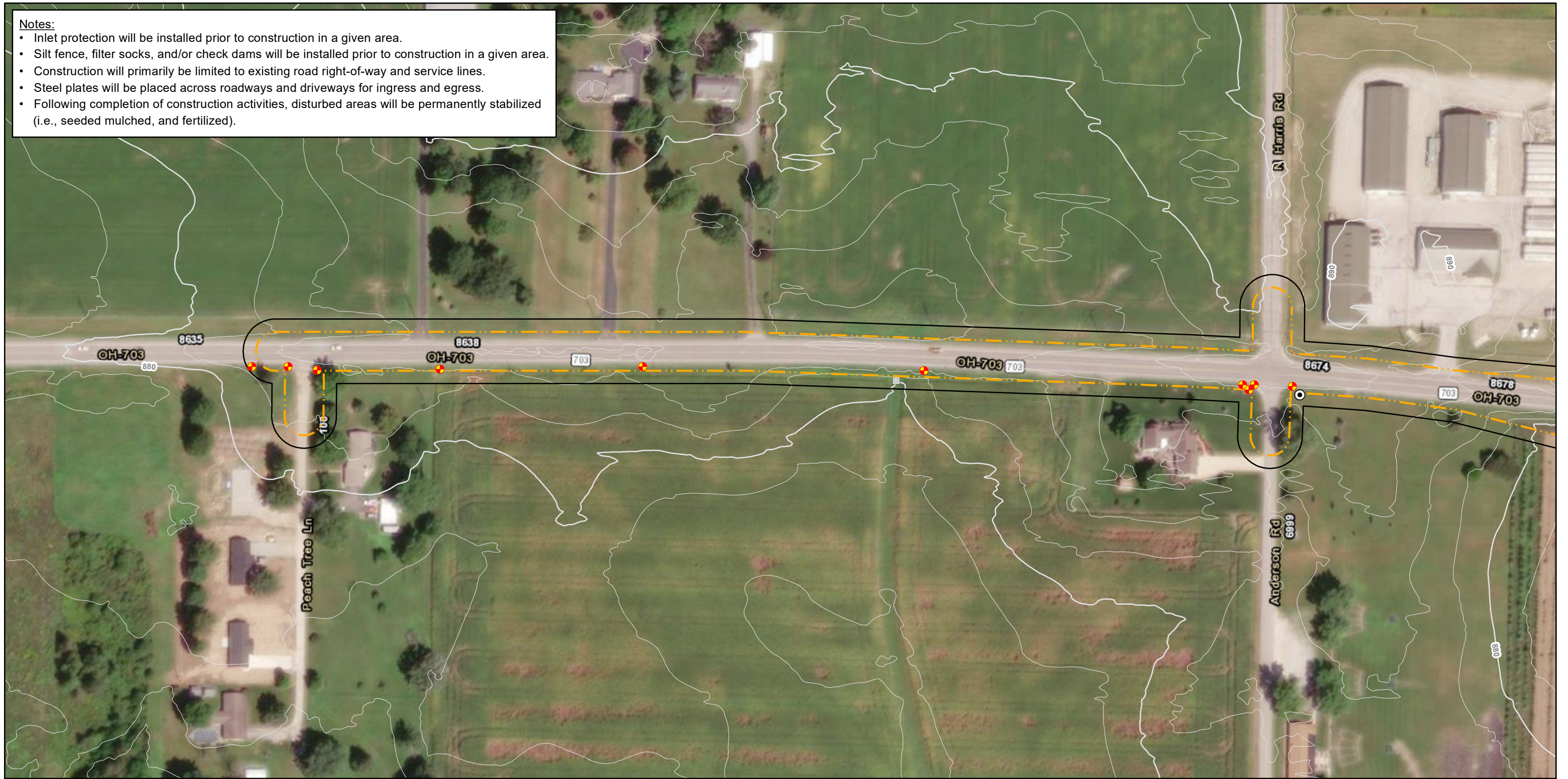
Figure C-1.01. SWPPP Map of Wetlands and Other Water Resources. PIR 2399 - Peach Tree S.R. 703.
