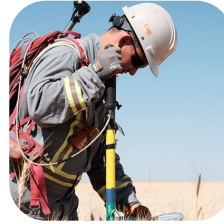
Close Interval Potential Survey (CIPS)
