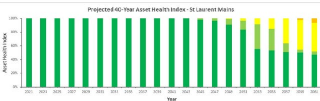
Figure 17: St. Laurent Pipeline Asset Health Index
