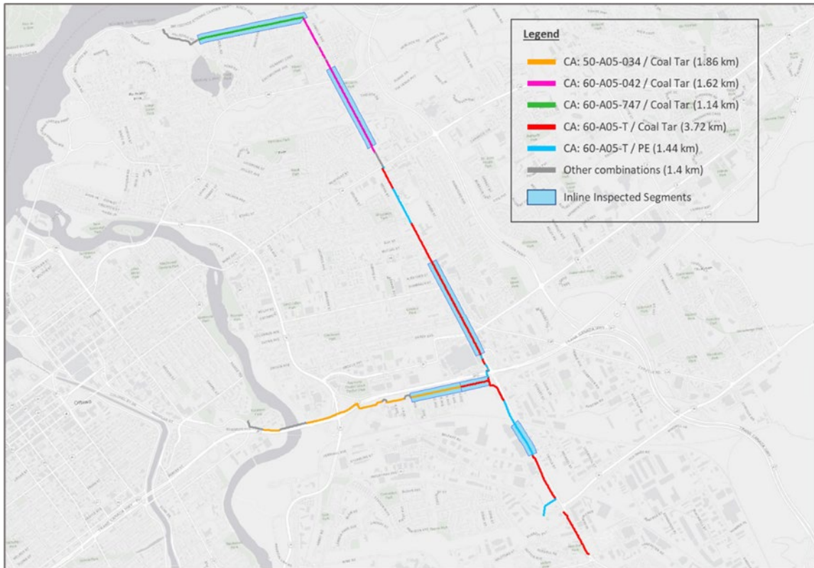
Figure 4: Pipeline Groupings with ILI Locations
